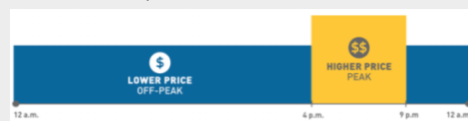
Figure 3: A visual example of a time-of-use rate schedule. (Pacific Gas and Electric, n.d.)
